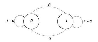
Figure 6 Illustration of the two-state, first-order Markov model<sup>10</sup>
