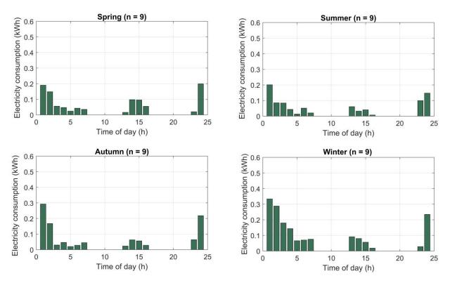
Figure 29 Average hourly electricity consumption heat pump hot water (night-rate & afternoon boost, per-occupant)
