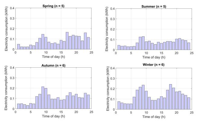
Figure 25 Average hourly electricity consumption uncontrolled standard electric hot water (per-occupant)
