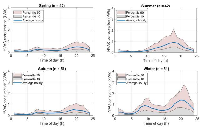
Figure 13 Illustration of the variability of the HVAC consumption across the associated fleet
