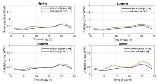
Figure E4 Underlying load profiles for customers with and without solar PV per season
