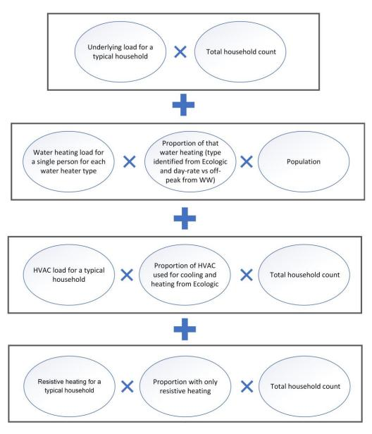
Figure 8 Illustration of the proposed method for scaling up load profiles
