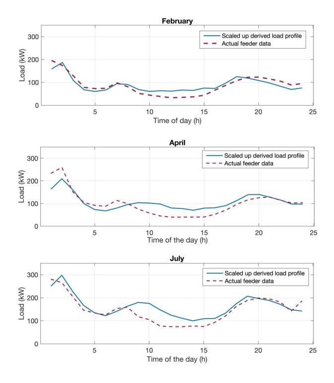
Figure E7 Scaled up derived typical load profiles benchmarked against actual feeder data for a summer month, a transition month, and a winter month – the sum of the three feeders
