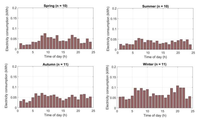
Figure 27 Average hourly electricity consumption uncontrolled heat pump hot water systems (per-occupant)
