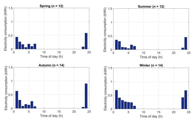
Figure 26 Average hourly electricity consumption controlled standard electric hot water (per-occupant)
