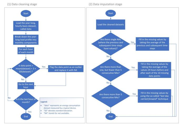
Figure 4 Sequential diagram of data cleaning and imputation techniques
