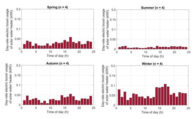
Figure 23 Average hourly electricity consumption uncontrolled electric boost elements SHW (per-occupant)
