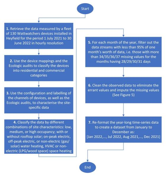
Figure 3 Flow chart of the overall method for deriving the load and sub-load profiles
