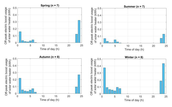
Figure 24 Average hourly electricity consumption controlled electric boost elements SHW (per-occupant)
