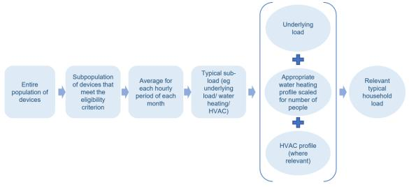
Figure E1 Overview of the method to derive the overall typical load profiles
