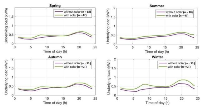
Figure 17 Underlying load profiles for customers with and without solar PV per season
