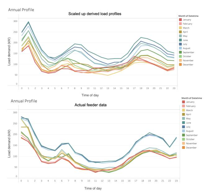
Figure 30 Scaled up derived typical load profiles benchmarked against actual feeder data over all months The sum of the three feeders of interest.
