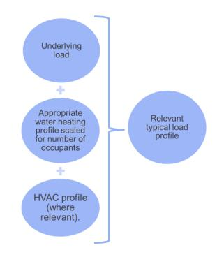
Figure 7 Process for building up the typical load profiles
